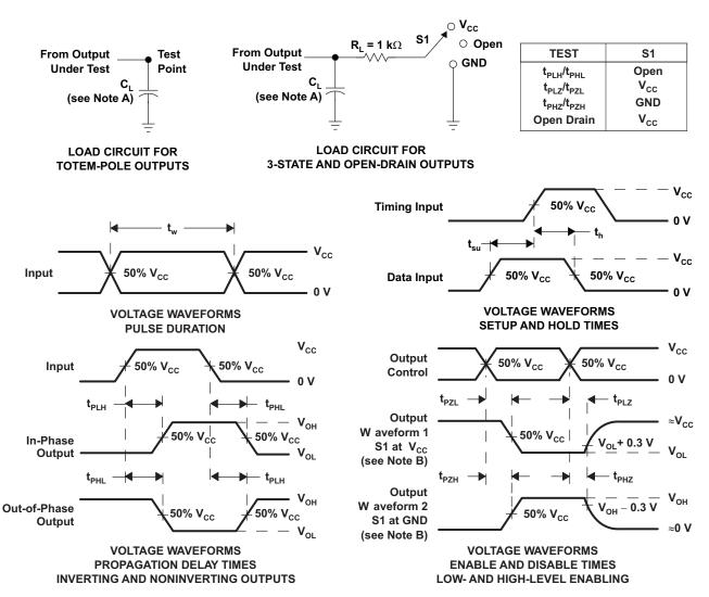
NOTES: A. C, includes probe and jig capacitance.
